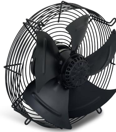
*W series axial fans are available from 200mm to 800mm diameter, both sucking and blowing type, 2-4-6 poles 230V - 50/60 Hz (single phase) and 230/380V - 50/60 Hz (three phase), with thermal protection and class B insulation.*
